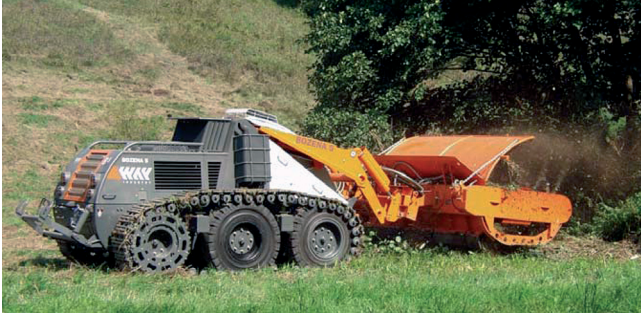
Fig. 48.7 Bozena teleoperated demining vehicle (Way Industry, Slovakia)
