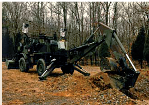
Fig. 48.14 Remotely operated excavator (courtesy of Oak Ridge National Laboratory)
