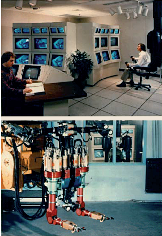
Fig. 48.11 Advanced servomanipulator system (courtesy of Oak Ridge National Laboratory)
